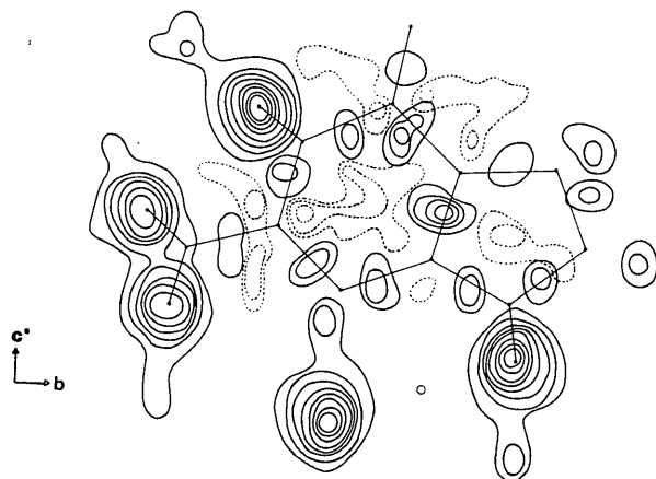
Fig. 3. Three-dimensional electron density difference map projected along [100]. Contours are at intervals of 0.1 e.Å -3 beginning at 0.1 e.Å -3 . Negative regions are shown by dashed contours.
